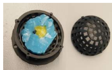
Figure 16: 3D printed scan container with “phantom” tissue sample used for testing
