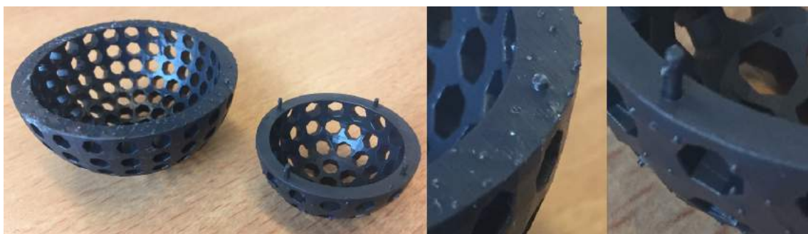
Figure 6: Remains of support structures added during input preparation
