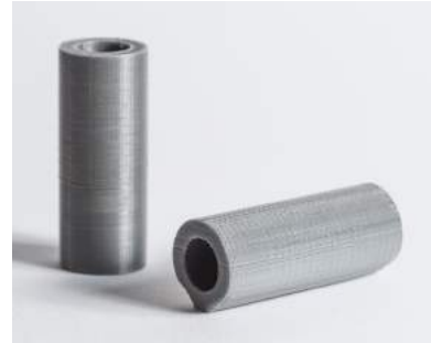
Figure 5: Visible staircase effect due to layered printing, which varying orientation within the 3D prints
