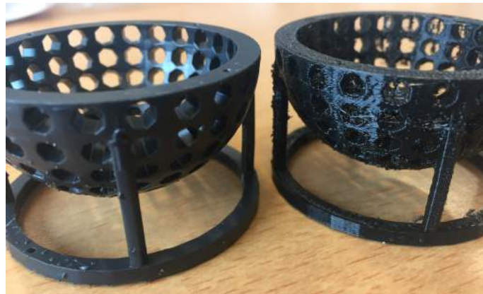
Figure 3: The influence of material choice: the exact same 3D model printed in two different materials (and with different printing techniques)
