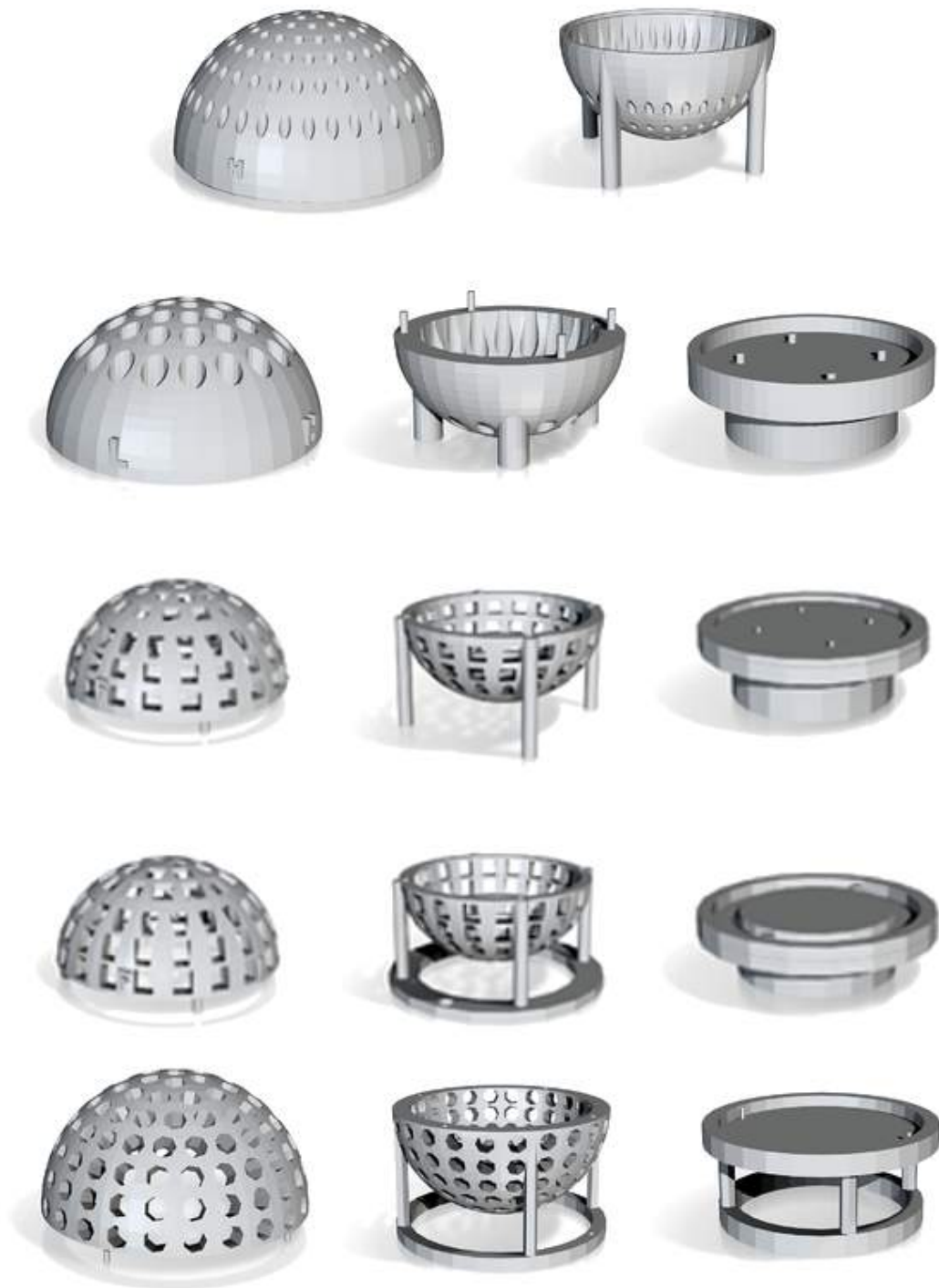
Figure 19: Evolution of the container design
