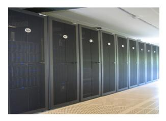
LISA Compute Cluster consists of several hundreds of multi-core nodes, running Linux. It is ideal for large-scale computations and suitable for both high-throughput computing as well as moderate parallel applications. User jobs are allocated to compute resources on node-level and automatically executed in a series of computer jobs (batch). Users are given a login, which enables immediate, 24/7 access to the service.
